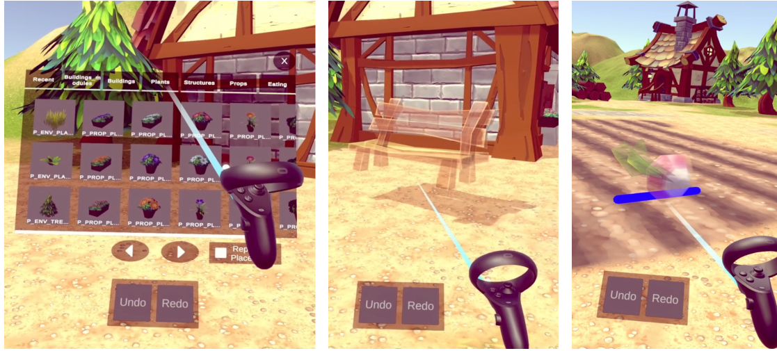
Figure 3.2: Left: Asset Menu with assets categorized in different tabs. Center: An asset that was selected through the menu is attached to the RayInteractor and being placed. Right: The rotation axis is visualized for the object being placed.
