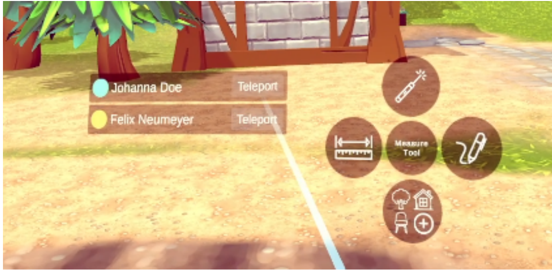
Figure 3.1: Left: User list with buttons for teleporting to other users. Right: Main menu with tool selection buttons for laser pointer, 3D pen, asset menu and measurement tool.
