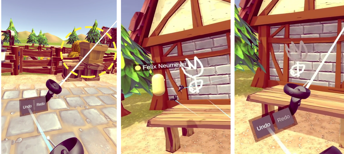
Figure 3.5: Left: Box on top is highlighted by a yellow tint as the next undo target. The yellow lines were added to clarify which box is highlighted, as it is hard to see in the screenshot. Center: Collaborator is drawing using the 3D Pen. Right: User is undoing the drawing made by the other user.
