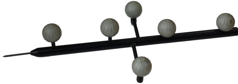
Figure 4.3: The MeaTool ART-target to measure positions in 3D at the tip.
