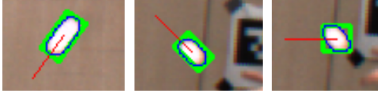
Figure 5.1: Length and radius estimation with minimum area rectangle. Rotated rectangle (green), direction from rectangle rotation (red) and FMO contour (blue). Left and middle images show a successful estimation. Estimation in the right image is incorrect due little elongation of FMO, even though slight elongation is visible.
