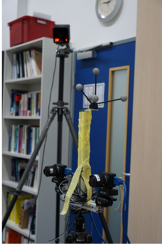
Figure 4.1: Two cameras mounted on a frame with an infrared (IR) tracking target above. A cable for hardware-synchronization connects both cameras. Tape to prevent IR-reflections. Background: one of four IR tracking cameras for validation and calibration.
